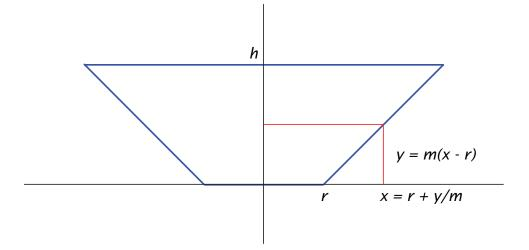
$$V = \int_0^h \pi x^2 dy = \pi \int_0^h \left(r + \frac{y}{m}\right)^2 dy = \pi \left(r^2 h + 2r \frac{h^2}{2m} + \frac{h^3}{3m^2}\right)$$
