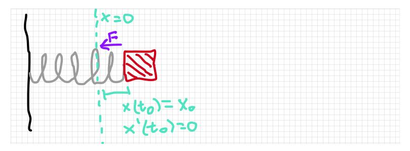
For an ideal spring, F = -kx. Remembering Newton's second law, F = ma = mx'', we get the secondorder homogeneous equation: mx'' + kx = 0. If we assume this equation will have solutions of the form
