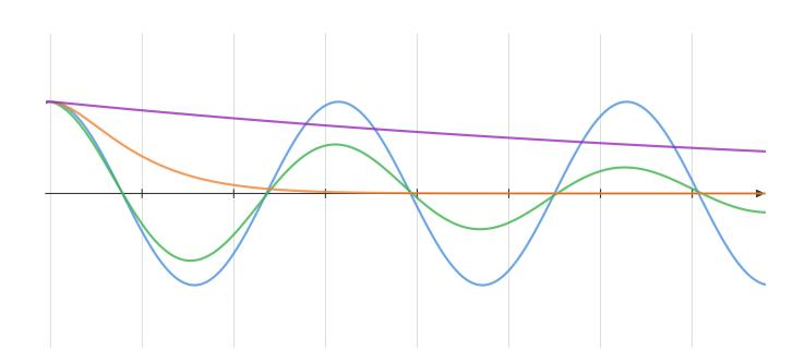
Purple: overdamped, Orange: critically damped, Green: underdamped, Blue: undamped
