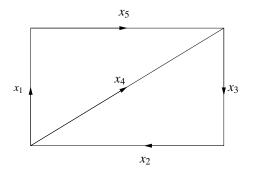
The flow into each corner must equal the flow out. This gives us the system of equations:
