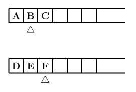
This can be simulated with a single tape (using bread crumbs to mark the position of both tape heads, as below:
