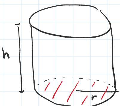
$$V = \text{volume} = \text{area of base} \times \text{height} = (\pi r^2) \times h = \pi r^2 h.$$
