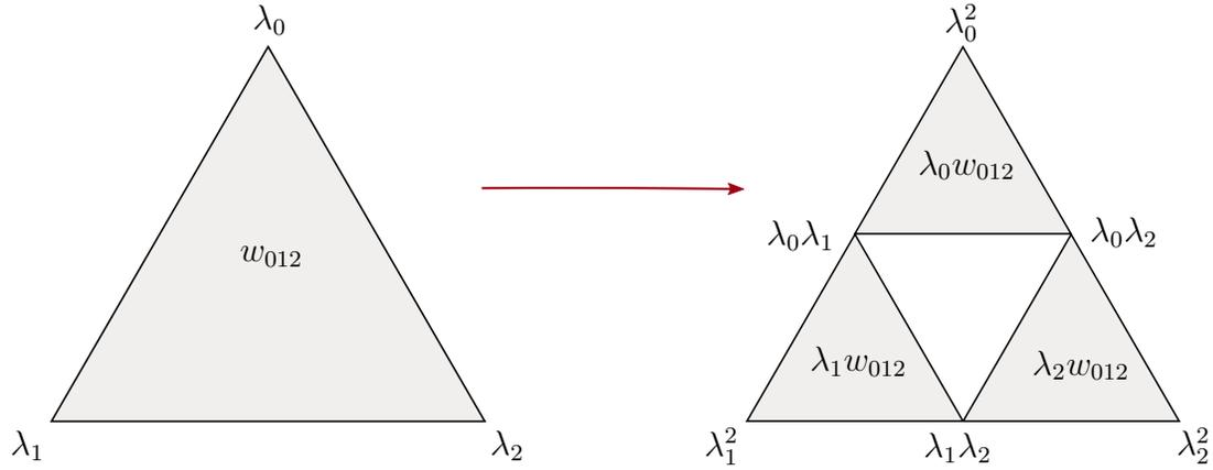
Figure 3.1: The Rapetti construction, as applied to a 2-simplex in  $\mathbb{R}^2$ . The Whitney 1-forms are not shown to reduce clutter. Note the hole formed in the center of the collection of small 2-simplices on the right.
